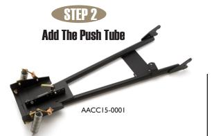
The Push Tubes are built of heavy-duty 11/2" steel tubing and are designed with maximum strength by triangulating the tubes. They also feature multiple swivel positions and four-way adjustment at the cutting edge. As always, these push tubes attach to the middle of the ATV conveniently with two quick pins.
