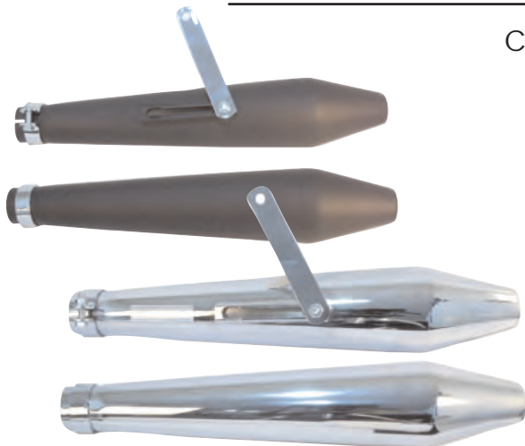
80-84032 CHROME FINISH 80-84033 FLAT BLACK FINISH CAFÉ MUFFLER AVAILABLE IN FLAT BLACK OR CHROME. 19" (483MM) OVERALL LENGTH. 1-3/4" INLET. STRAIGHT THROUGH PERFORATED CORE TYPE BAFFLE. SLOTTED CHANNEL TYPE MOUNT FITS RIGHT OR LEFT. 1-5/8", 1-1/2" AND 1-3/8" (3 PIECE) REDUCER KIT INCLUDED
