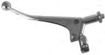
32-64452 Ball end clutch lever for 1" handlebar with cam adjuster Doherty type 217 replica
