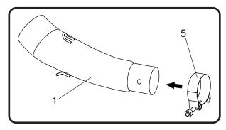
2. Install (No. 4) *HT SHLDTRS*, muffler clamp heatshield onto (No. 3) *YM7M-MPCA(X)*, muffler clamp.
