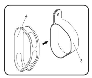
3. Slide (No. 3) *YM7M-MPCA(X)*, muffler clamp over Yoshimura muffler.
