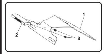
Secure (No. 1) 13320-FEBKT, fender eliminator bracket to frame using (No. 6) M6X16BHS, bolts and the stock nuts.
