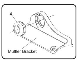
2. Install (No. 5) *ALS-003,* aluminum spacer into (No. 4) *Z1022,* rubber grommet as shown.
