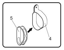
6. Slide (No. 4) YM7M-MPCA(X), muffler clamp over (No. 3) muffler. Secure muffler to the outside of the muffler mount using the stock bolt, washer, and nut.
