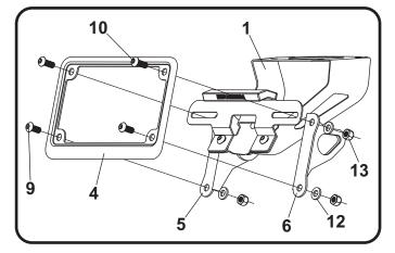
7. Install assembled fender eliminator bracket using (No. 11) *M6X16H*, 6mm hex head bolts, (No. 12,13) *6MMWASHER and 6MMLN*, washers and nuts.
