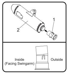
Install Yoshimura muffler/tailpipe assembly over the stock header outlet and align muffler bracket to muffler mount. Secure using (No. 3) M8X60FS, 8mm flat head screw, stock muffler mount washer and (No. 4) 8MMNUT, 8mm flange nut. Do not torque at this time.
