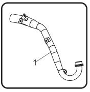
2. Install (No. 4) *HT SHLDR77,* muffler clamp heat insulator onto (No. 3) *12130-MPCX,* muffler clamp and trim excess heat insulator.
