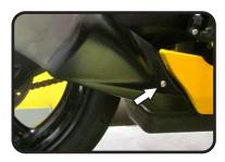
Loosen muffler exhaust clamp and while securely supporting the stock muffler assembly, remove muffler mount bolt and carefully remove the stock muffler assembly by sliding toward the rear of motorcycle.
