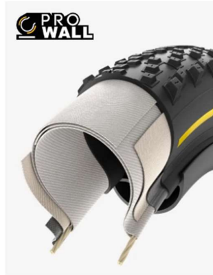
PRO WALL The reinforced MTB casing developed for cross-country, marathon, downcountry and light trail application
