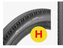
The Cinturato<sup>™</sup> Gravel **H** is a gravel-specific tyre designed for compact terrain and the hardest surfaces. The tread features low, tightly packed knobs and an elevated ability to adapt to the terrain, offering a large contact area and therefore excellent feeling while riding. Cinturato<sup>™</sup> Gravel **H** is a highperformance tyre with unique characteristics of grip in all weather conditions, both wet or dry, plus a high level of puncture protection.
