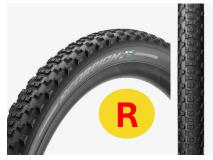
Rear wheel-specific tyre with a special tread pattern engineered for traction and braking grip. The Scorpion<sup>™</sup> XC **R** is the ideal rear tyre for everyday training. Medium profile tread design with added traction and durability for uncompromising performance over a variety of terrains. The Scorpion<sup>™</sup> XC R is the optimal rear tyre when paired with a Scorpion™ XC M at the front
