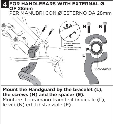
**Mount the Handguard by the bracelet (L), the screws (N) and the spacer (E).**
